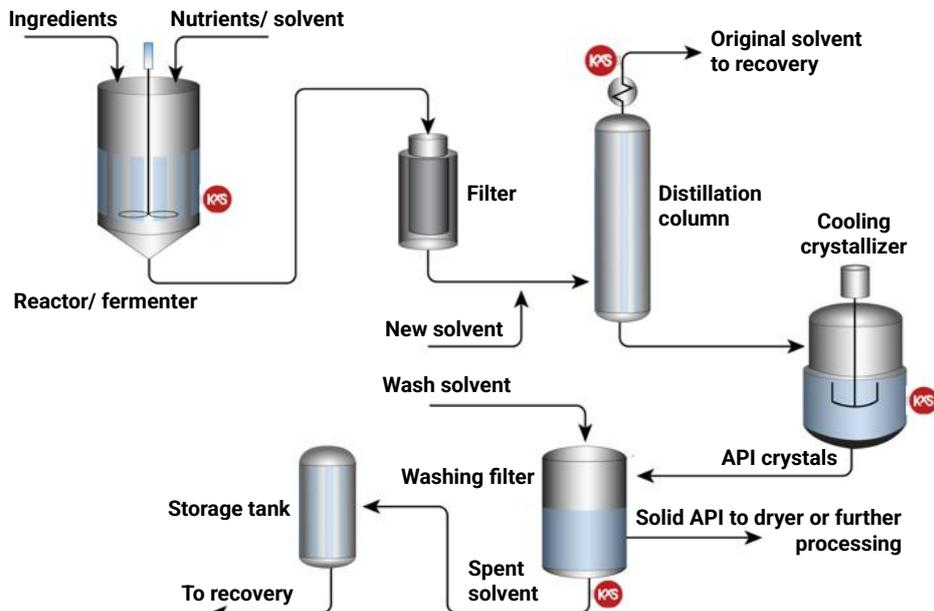
KxS refractometer provides real-time monitoring of RI to track the degree of conversion and detect the reaction endpoint. In bioreactor fermentation, it supports nutrient feeding control and metabolic monitoring.
