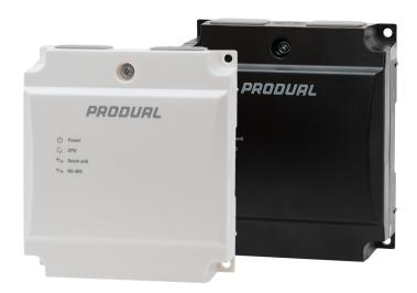
Produal Proxima<sup>®</sup> CU-LH control unit is designed especially for more advanced room and zone control applications that demand more functionality than traditional controllers. The control unit supports the Modbus RTU communication protocol. The control unit is built on the Produal PUMP<sup>®</sup> (Produal unified and modular platform).
