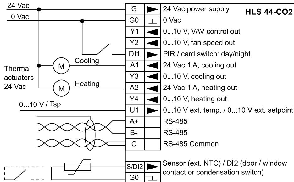
The maximum triac output current is 1 A. For example, up to three A 40405 thermal actuators can be connected to one output. Then the total current consumption doesn't exceed 1 A.
