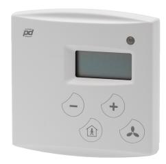
HLS 44-SE is a versatile room controller for room-specific temperature and variable air volume (VAV) control. With the standard RS-485 connection, you can connect the controller to any system that supports the Modbus RTU protocol. The bus is galvanically isolated from the other electronics in the controller.
