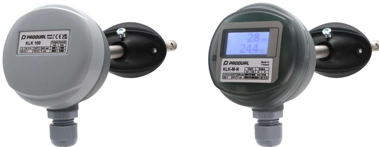
The KLK duct humidity transmitters measure relative humidity and temperature inside ventilation ducts. They are designed for high- and low-humidity applications in non-condensing environments. These transmitters have a broad humidity measurement range and a wide temperature measurement range. You can set a custom measurement range (low and high limit) separately for both humidity and temperature measurement.
