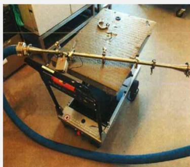
KxS Technologies commissioned a EHEDG Authorized Testing Laboratory to perform the cleanability test method (EHEDG Doc. 2) of food contact faces of the inline Brix monitor.
