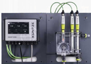
❖ Water Quality Monitoring System (pH, Conductivity, Turbidity, Total chlorine, Free Chlorine, Sulfate & Temp. Measurement)
