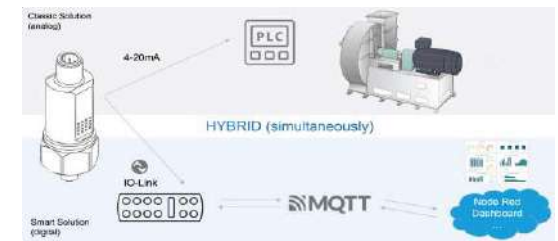
Smart Vibration Sensors (IO-Link)
