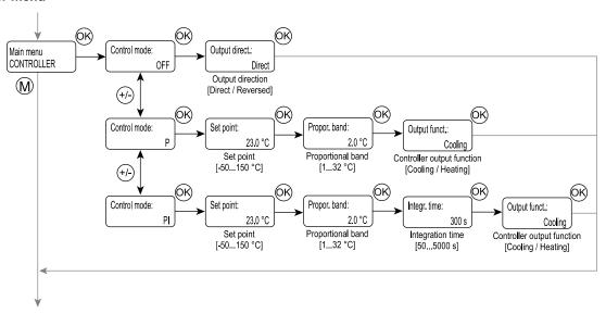
In controller menu the temperature output can be changed to controller output. You can also change the controller settings in the menu.
