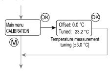
The temperature measurement can be tuned through the calibration menu. The temperature value can be adjusted by 0,1 °C steps. ML-SER tool display shows the tuned value.
