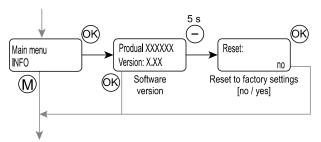
The info menu can be used for checking the software version, and resetting to the factory settings.
