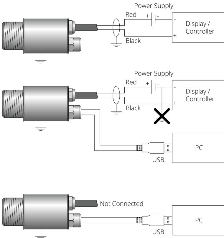
Note: The sensor must be grounded at only one point, either the cable shield or the sensor housing.
