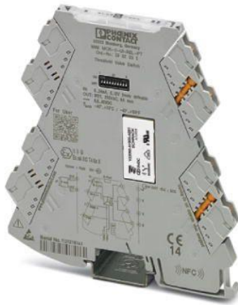
Figure 44 Limit value switch. Universally configurable limit value switch with PDT relay output and plug-in connection technology for switching analog limit values. Configurable via DIP switch or software. Push-in connection technology, standard configuration.
