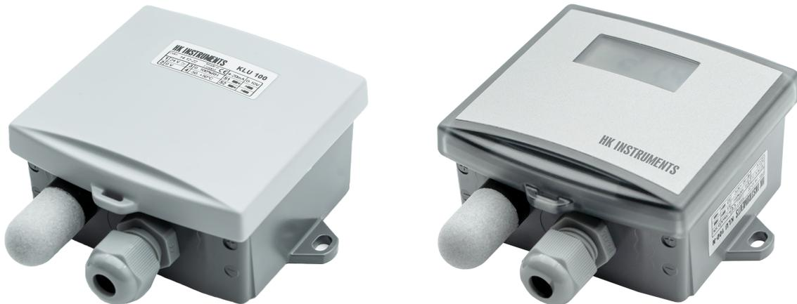
KLU 100 temperature and humidity transmitters are designed for outdoor applications. The transmitter has a capacitive sensor that detects relative air humidity and an NTC10 sensor for temperature measurement. A sintered plastic filter protects the sensor elements.
