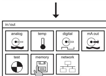
If the datalog add-on is activated, four symbols appear. In the menu LOG PARA you define which parameters you want to log. In LOG SET you define interval and log mode, and view the log status.
