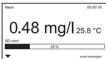
This adds a status bar indicating the remaining storage space on the SD card.
