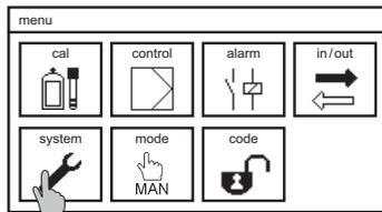
Select the symbol SYSTEM in the main menu, and in the submenu the symbol RESET.
