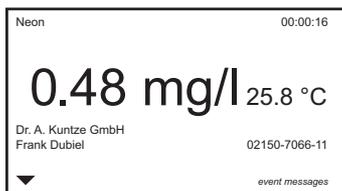
This adds the contact data that is stored in the submenu SYSTEM → CONTACT.
