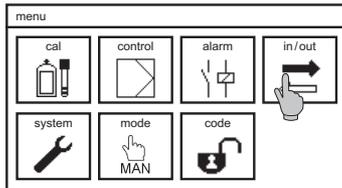
Select the symbol IN/OUT in the main menu and then the symbol ANALOG. A submenu opens, showing four drop-down lists.
