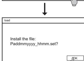
The display shows the name of the file that will be loaded. The name consists of the parameter and the date. Acknowledge with OK.
