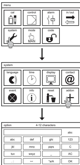
To activate add-ons, select the symbol SYSTEM in the main menu, and in the submenu the symbol ADD-ON.
