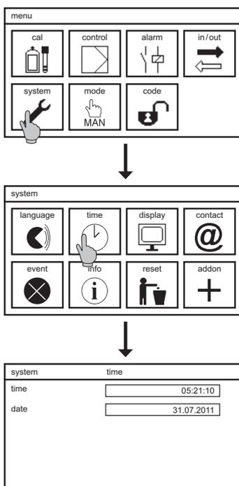
To set the internal clock, select the symbol SYSTEM in the main menu, and in the submenu the symbol TIME.
