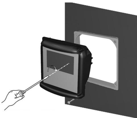
Place the instrument inside the frame and secure it with the M4 x 25 screws. Tighten the screws until the instrument is firmly fixed.
