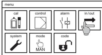
Select the symbol IN/OUT in the main menu and then select the symbol mA OUT. Here you can set the following parameters:
