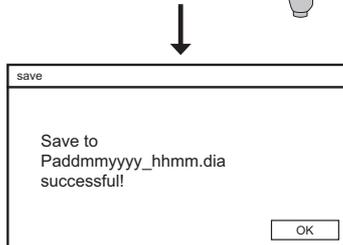
The display shows the name of the created file. The name consists of the parameter and the date. Acknowledge with OK.
