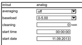
Select the symbol IN/OUT in the main menu, and in the submenu the symbol ANALOG. Subsequent to the usual parameters you find four more parameters that concern the cleaning function:
