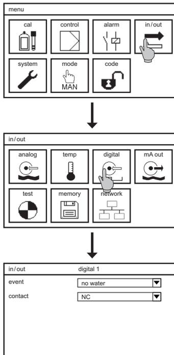
In the entry-level version, the Neon® instrument has one digital input. All settings concerning the digital input(s) are found in the submenu IN/OUT → DIGITAL. If you have two digital inputs, separate symbols will appear for them.
