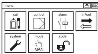
Press the triangle on the left side of the bottom line of the desktop to enter the main menu. In the main menu, select submenus by touching the corresponding symbols.
