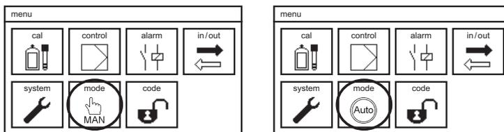
In the AUTO mode the controller is active and operates the relays and/or current outputs and ultimately the connected actuators. Manual operation of the relays and current outputs via the test function is not possible.
