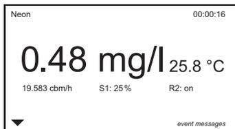
This adds the calculated flow rate, the controller output in %, and the status of relay 2.
