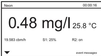
Below the measured values the flow rate, the controller output in % and the status of relay 2 are displayed.
