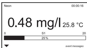
This adds an analog bar indicating the controller output for set point 1 or 2, respectively, in %.
