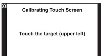
To calibrate the touch screen, select in submenu SYSTEM → DISPLAY the symbol TOUCH CAL to start the calibration. The touch screen calibration texts are available in English only.
