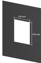
Prepare an opening of 138 x 138 mm. Clip the installation frame into the opening.
