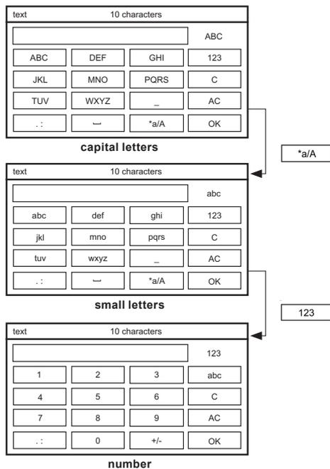
**Note** With numerical parameters, the keyboard automatically shows only numbers.
