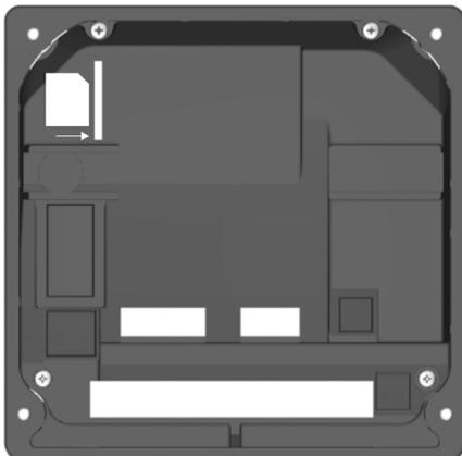
Press the SD card – with angled edge top right – into the slot until it is into place.
