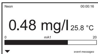
This adds an analog bar indicating the mA output of output 1 or 2, respectively.
