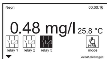
Below the measured values the configuration and status of the relays are displayed, and a button appears with which you can change the operation mode.
