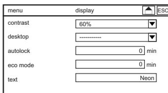
In submenus you will find on the left side the parameters and on the right side the corresponding settings. If the submenu contains more parameters than can be shown, a scroll bar on the right side gives access to the parameters currently not shown.
