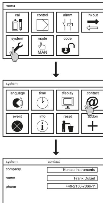
Select in the submenu SYSTEM the symbol CONTACT. For each field a keyboard opens to enter the name or number.
