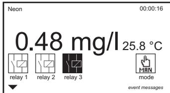
This adds the status of all three relays and the mode. Active relays are shown white on black, and the symbol shows whether the relay is open or closed. See relay 3 in the example shown.
