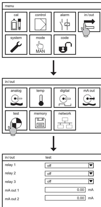
Set the mode to manual. Select the symbol TEST in the submenu IN/OUT.
