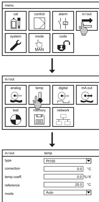
All settings concerning temperature measurement and compensation are found in the submenu IN/OUT → TEMP. Select the symbol IN/OUT in the main menu, and TEMP in the submenu.
