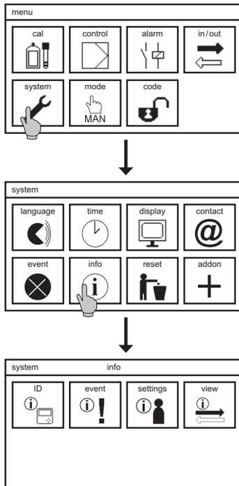
The submenu INFO is found in the submenu SYSTEM. It contains four symbols:
