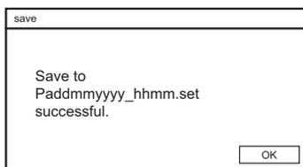
The display shows the name of the created file. The name consists of the parameter and the date. Acknowledge with OK.
