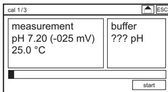
> Put the pH sensor in the first buffer solution and press START. Default values for the buffer solutions are pH 4 and pH 7. If you want to use other buffer solutions, you have to change the calibration settings.
