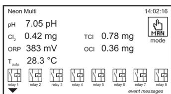
This adds the status of all relays and the mode. Active relays are shown white on black, and the symbols show whether the relay is open or closed.
