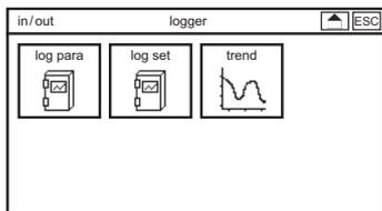
In the menu LOG PARA you decide which parameters are logged, in LOG SETTINGS you define interval and log mode and view the status. In TREND you can see a graphical display of the measured values over the last 2h, 24h or 72h.
