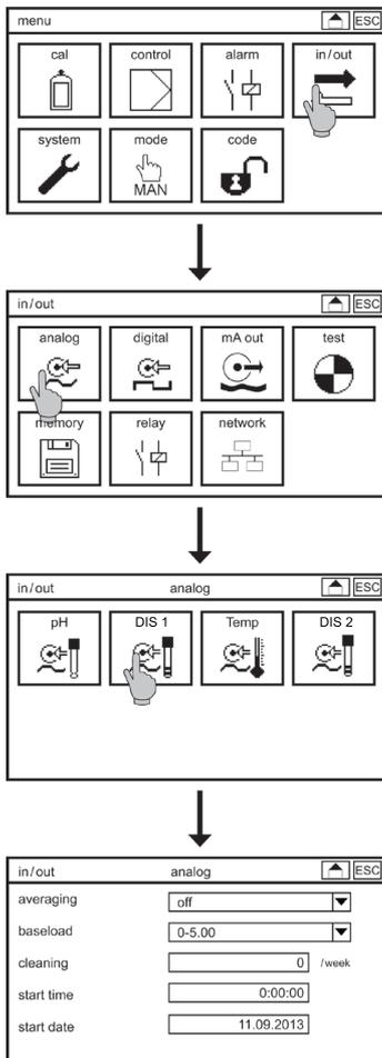
Select the symbol IN/OUT in the main menu, and in the submenu the symbol ANALOG, and then DIS 1. Subsequent to the usual parameters you find four more parameters that concern the cleaning function:
