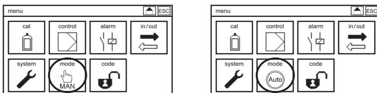
In the AUTO mode the controller is active and operates the relays and/or current outputs and ultimately the connected actuators. Manual operation of the relays and current outputs via the test function is not possible.
