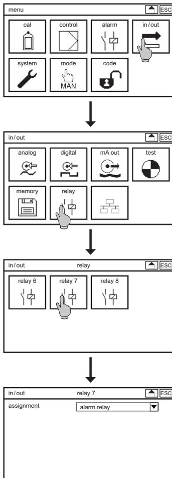
Select in the menu IN/OUT the symbol RELAY. In the submenu you can define for relays 6, 7 and 8 whether they work as alarm relays or have different functions.
