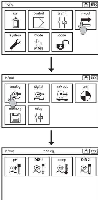
In the submenu ANALOG you can choose between the activated measuring inputs: pH, DIS 1, temperature, conductivity or DIS 2.
