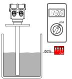
Total empty-fill of container is not necessary, any level can be calibrated using external multi-meter.
