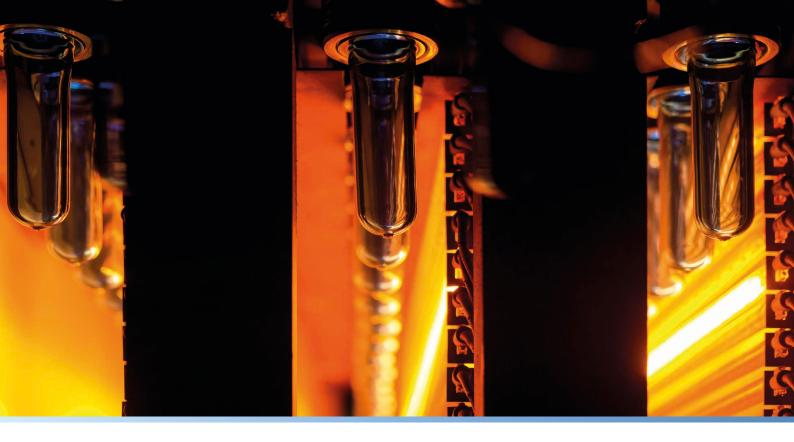
Infrared temperature sensors are helping to provide consistent product quality in the high-speed process of injection blow moulding.
